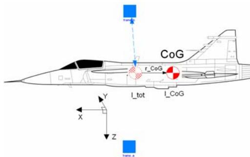
**Figure 4.** Aircraft with variable center of gravity and mass moment of inertia.
