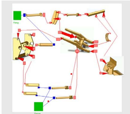
**Figure 3.** Left: 3D view of wheel loader mechanism created in a 3D mechanical CAD system. Right: Connected components from the wheel-loader library, forming a model of a wheel-loader mechanism.
