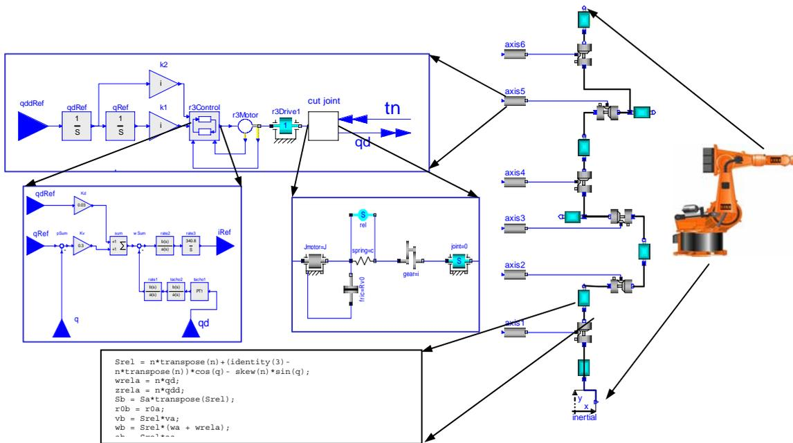
**Figure 1.** Hierarchical model of an industry robot, including components such as motors, bearings, control software, etc. At the lowest (class) level, equations are typically found.
