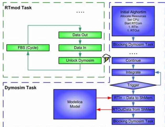
Figure 2: Functional overview of the Modelica real-time interface
