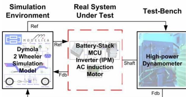
Figure 5: Electric two-wheeler hardware-in-the-loop simulation
