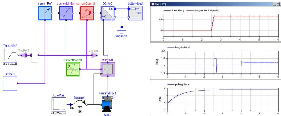
Field Oriented Control of an asynchronous induction machine drive – analysis of transient behavior
