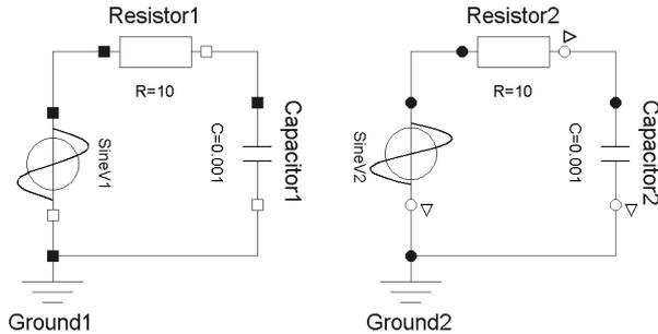
**Figure 13:** Schematic of domain-switching example; left: always within time domain, right: switching from time domain to phasor domain (T-P) and reverse (P-T)
