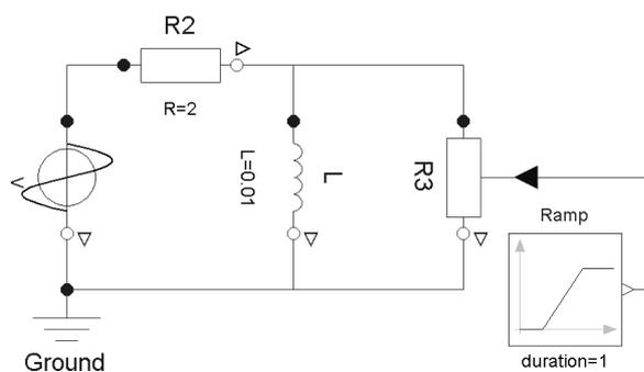
**Figure 6:** Example circuit
