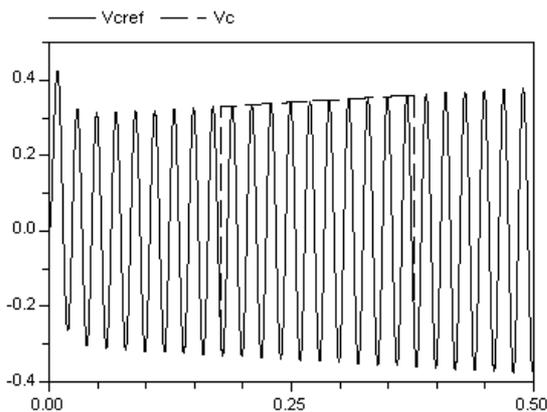
**Figure 14:** Voltages;  $V_{\text{cref}}$ : always in time domain,  $V_c$ : switching T-P and P-T (showing amplitude in P-domain)
