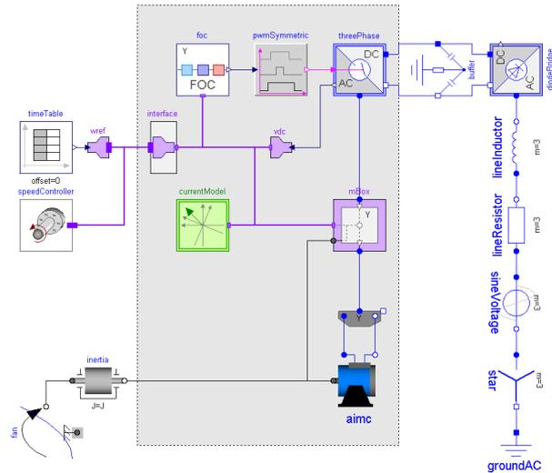
Figure 14: Case C; electrical transients and switching effects simulation of the speed controlled fan drive with elementary SED models.
