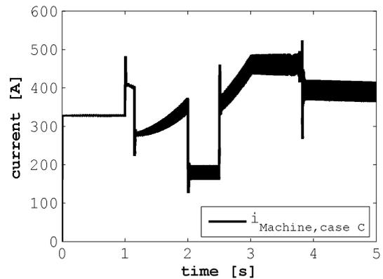
Figure 15: RMS value of the stator phase current of the machine in case C.
