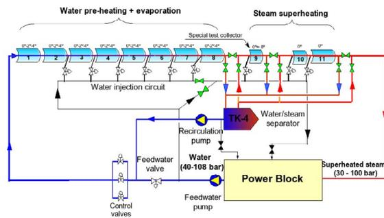
Figure 2: Schematic diagram of DISS facility at PSA
