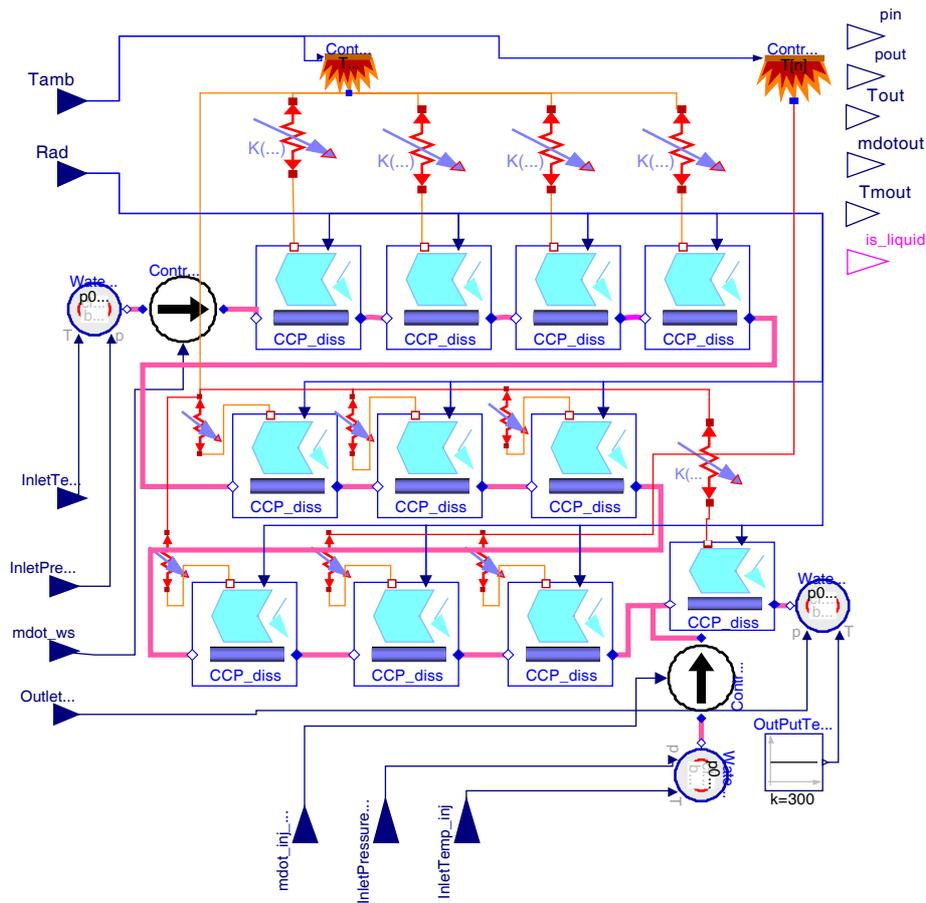
Figure 4: Modelica model of DISS plant in *once-trough* configuration.
