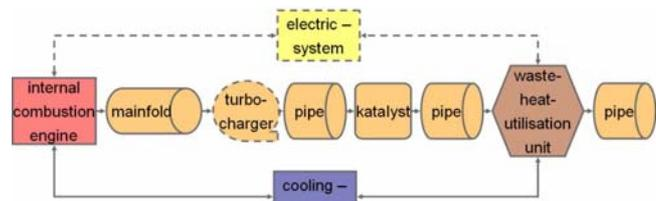
Figure 3: Scheme of exhaust system
