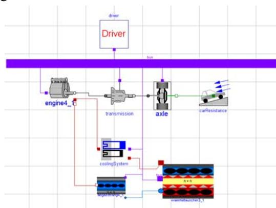
Figure 1: Object diagram of the PowerTrain vehicle model
