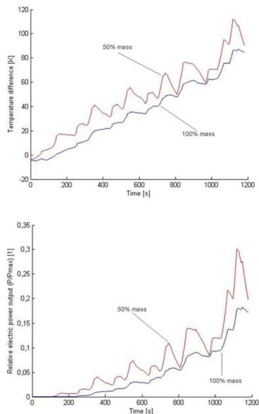
**Figure 8: Top: Temperature difference between hot and cold side of the thermoelectric device with 50% (red) and 100% (blue) mass over the NEDC; bottom: Relative electrical power output of the thermoelectric device with 50% mass (red) and 100% mass (blue) over the NEDC.**
