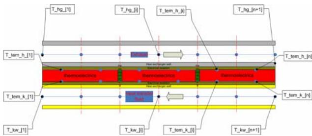
Figure 4: Scheme of the waste-heat-utilization-unit.
