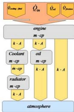
Figure 2: Thermal engine model with 4 masses
