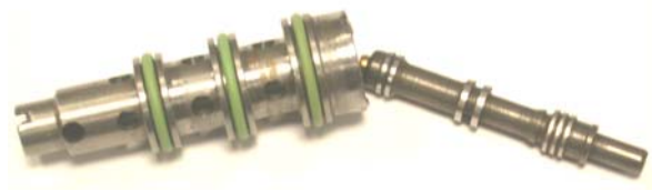
Figure 2: Typical hydraulic spool
