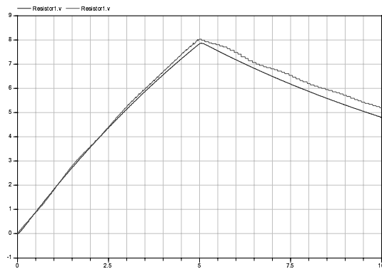
Figure 6: Plot of voltage over the resistor component, T_{tlm}=0.1 , interval length=0.01s
