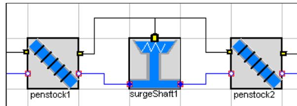
**Figure 6. Example of the interconnected penstocks and surge tank**
