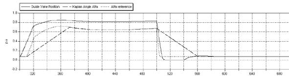
**Figure 16: Guide vane position, Kaplan angle and angle reference**
