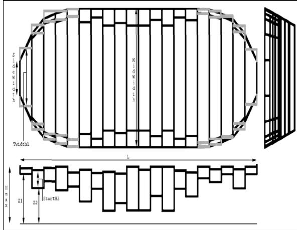
**Figure 3. Parameters for dimensioning of the reservoir**
