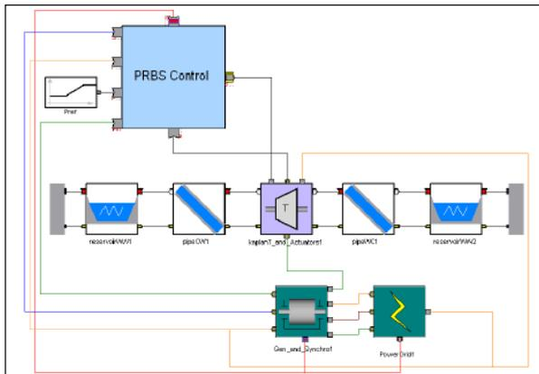
Figure 11. Model of a complete hydro power plant
