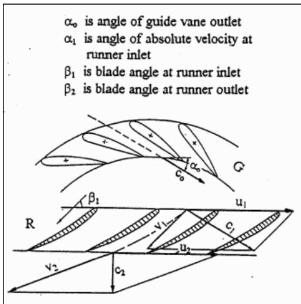
**Figure 10: Angles of Kaplan water flow velocities**
