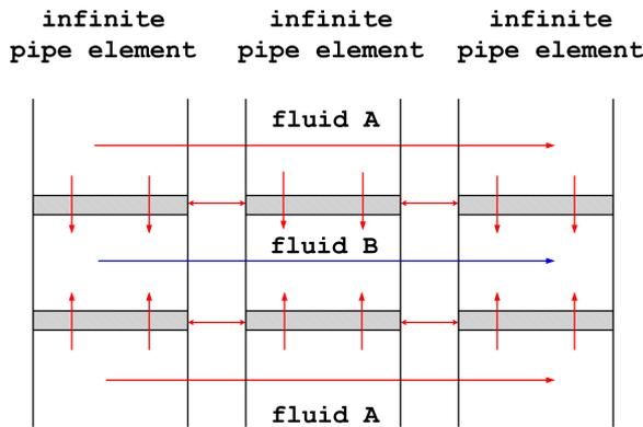
Figure 7: Scheme of a parallel tube heat exchanger
