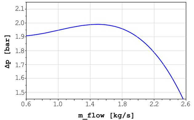
Figure 2: Characteristic of the centrifugal water pump with losses
