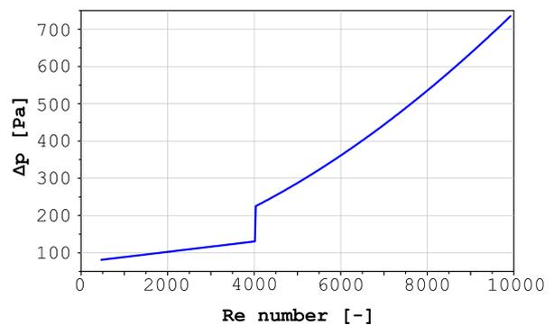
Figure 4: Pressure drop in pipes versus flow velocity
