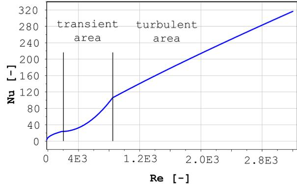
Figure 5: Nu number versus increasing flow velocity
