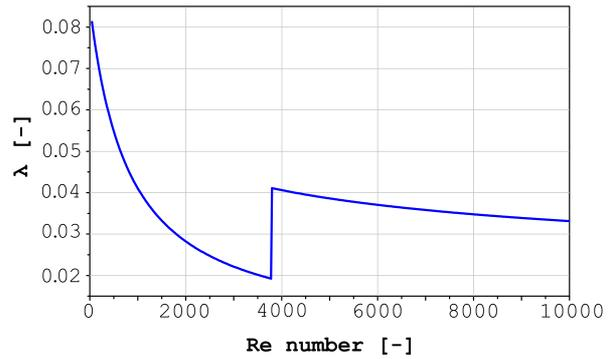
Figure 3: Coefficient of friction versus different flow types
