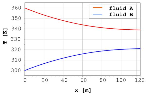
Figure 9: Temperature distribution inside the heat exchanger
