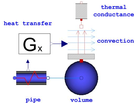
Figure 6: Model of an infinite small pipe segment
