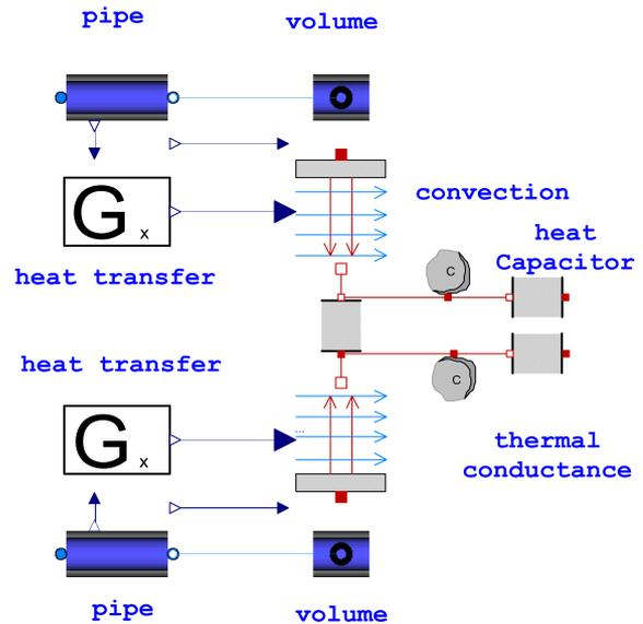
Figure 8: Model of a segment of a parallel heat exchanger
