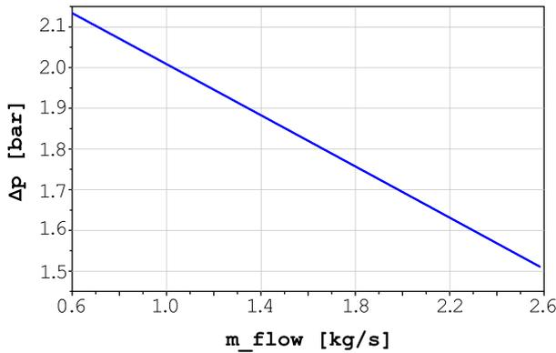
Figure 1: Characteristic of an ideal water pump
