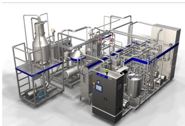
Figure 1. A typical dairy process-line for pasteurization.
