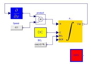
Figure 3: MOL model of linear advection equation
