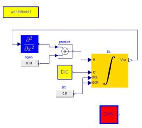
Figure 1: Model of 1D diffusion equation in PDELib
