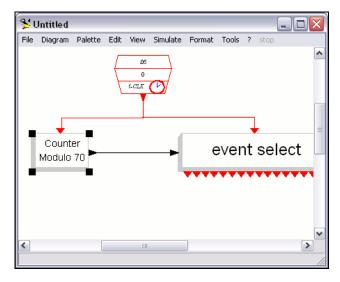
An alternative procedure consists of constructing a vector of time instants where events occur over a single period (in this case [0,2,3,4]) and generate events using independent event sources corresponding to time instances which, modulo 6, are mapped to the elements of this vector.
