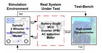
Figure 5: Electric two-wheeler hardware-in-the-loop simulation
