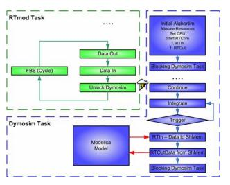
Figure 2: Functional overview of the Modelica realtime interface
