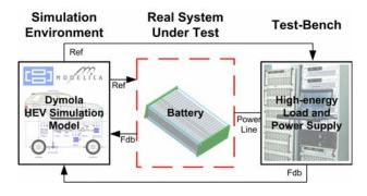
Figure 4: HEV hardware-in-the-loop simulation
