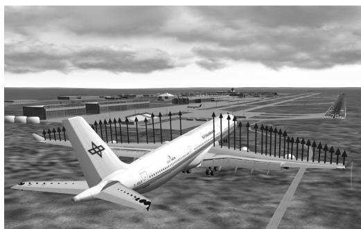
Figure 6: 3D-stereo visualisation of aircraft flight and structural dynamics, and aerodynamic loads
