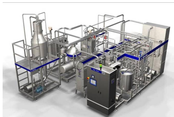
Figure 1. A typical dairy process-line for pasteurization.
