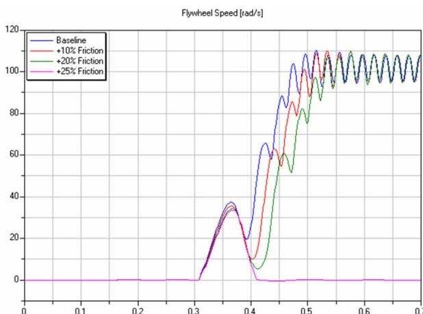
Figure 7: Friction Sensitivity
