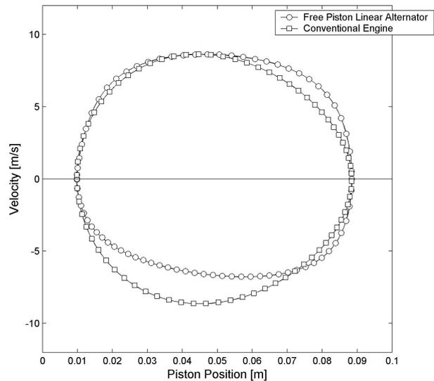
Figure 6: Comparison of piston velocities for crank shaft engine versus a free-piston linear alternator
