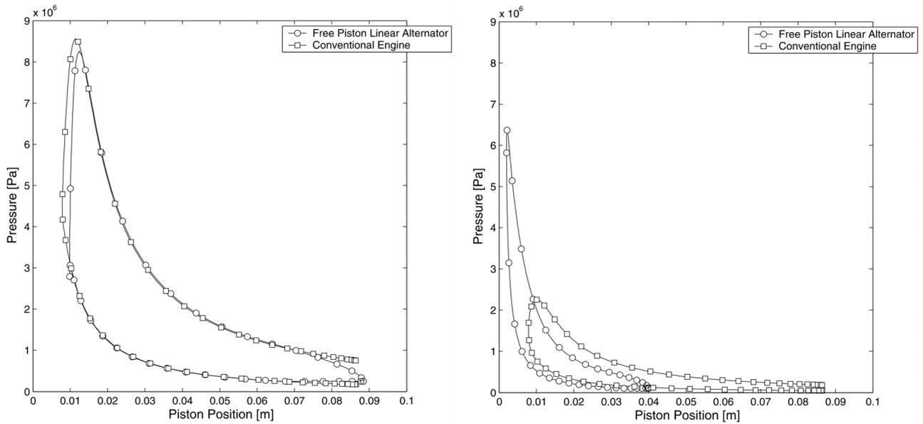
Figure 7: Comparison of combustion pressure at full (left figure) and part (right figure) load conditions for a crank shaft engine versus a free-piston linear alternator
