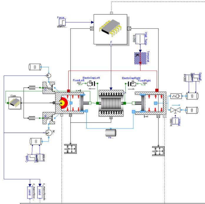
Figure 2: Modelica assembly of free-piston linear alternator
