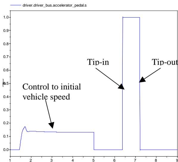
Figure 8: Accelerator pedal profiles
