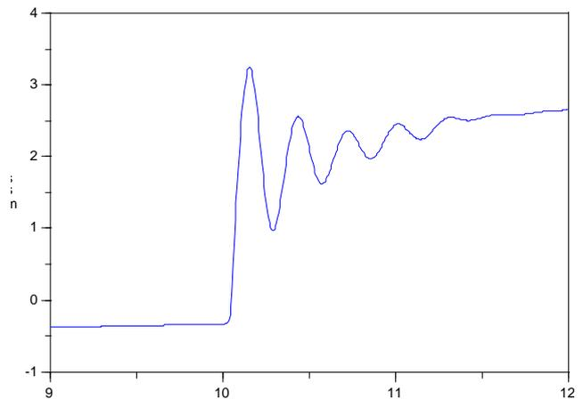
Figure 2: typical longitudinal acceleration due to a tip-in manoeuvre
