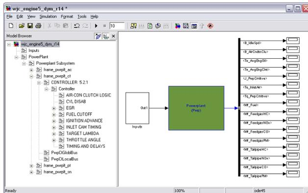
**Figure 3:** Simulink model created for automatic translation
