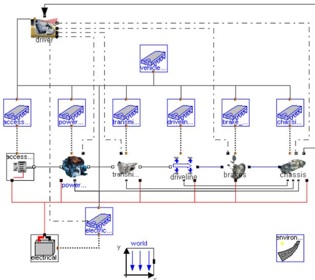
Figure 1: Top level of the Modelica VMA
