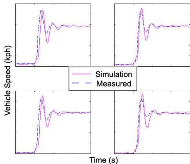
**Figure 11:** Correlation of tip-in results at various engine speeds in second gear
