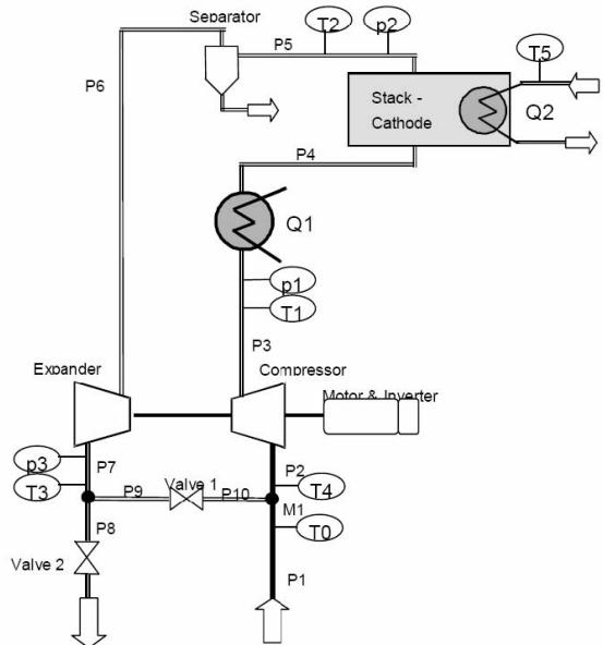
Figure 1: Sketch a the fuel cell subsystem to simulate
