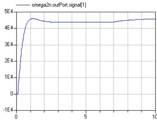
Figure 8: Simulation of system startup: angular velocity of common shaft
