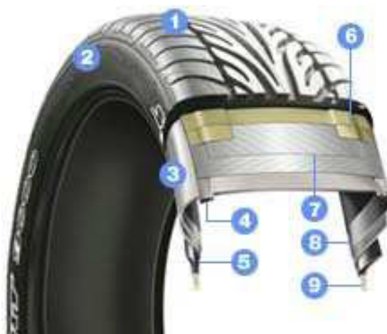
Figure 1: The tyre construction of a normal passenger car tyre. 1 - tread, 2 - sidewall, 3 - radial cord, 7 - belt, 9 - bead.
