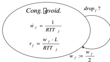
Figure 4: Simplified model of congestion control in TCP.
