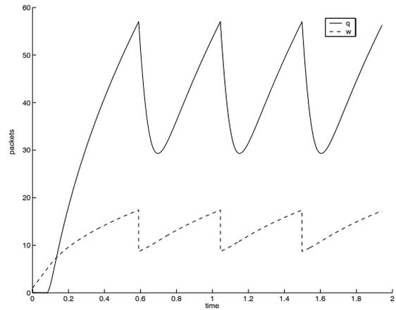
Figure 5: Illustration of congestion avoidance for a network with a single router. When the queue  $q$  (solid) exceeds  $q_{max} = 57$ , one packets is dropped. TCP reduces accordingly the window  $w$  (dashed) by a factor two. Note the characteristic shape of  $w$  with intervals of approximately linear growth and periodic jumps.
