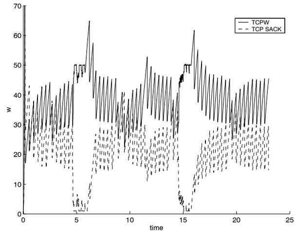
Figure 8: Simulation of the system in Figure 6. The windows size for TCP SACK is considerably reduced when the wireless link is losing a lot of packets (at about  $t = 5$  and  $t = 15$ ), while TCPW is able to cope with the losses very well.
