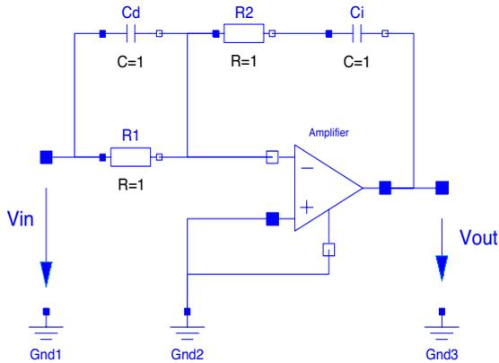
**Figure 4:** PID circuit
