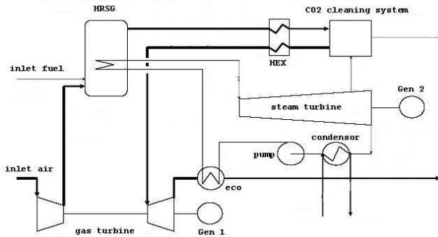
Figure 1: Sargas process flow sheet.
